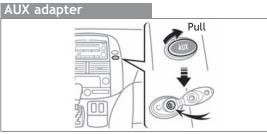
By inserting a mini plug of a commercially available component into the AUX adapter, you can listen to music from a portable audio device through the vehicle's speaker system.
